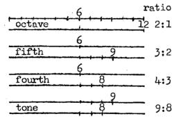
The numbers represent the positions of the bridge for each interval on the Pythagorean monochord. For instance, in the first example the octave interval is produced by doubling the length of string permitted to sound, hence the ratio 2:1. For convenience the line representing the string has been divided into twelve equal segments.
